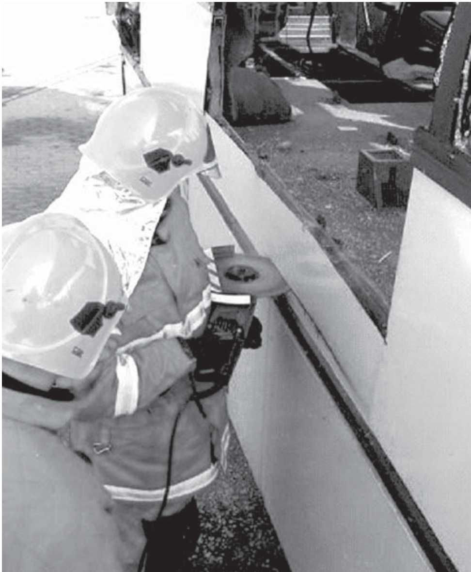
Cutting an opening of a passenger bus for rescue by Danish Rescue and Fire Fighting School Tinglev in June 2004
