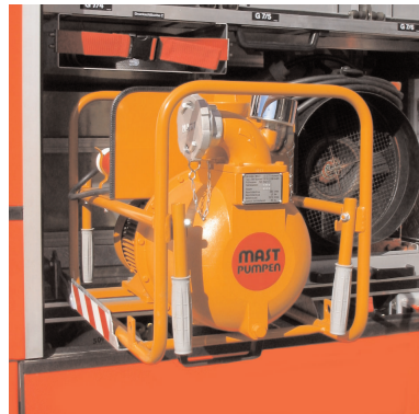
Accommodation of the MAST-ex-proof transfer pump in the fire-fighting vehicle.
