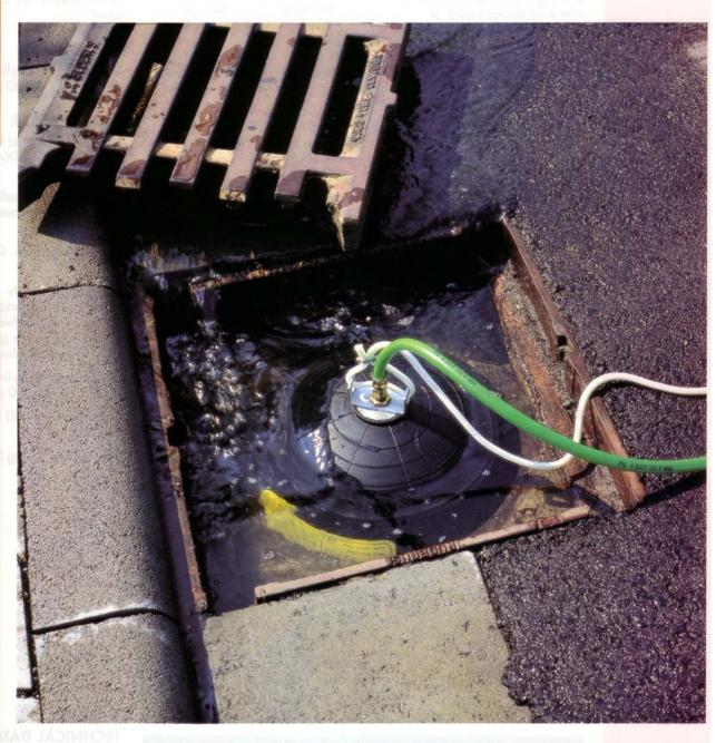
Toxic liquids spilling from road tanker crashes invariably take the fastest way into the sewer network. Polluted fire-fighting water poses a similar threat. Both endanger the groundwater and the environment. Yet there is a fast and easy remedy: the Vetter Compact Gully Sealing
