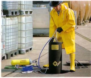
Vetter Sealing Bags are used to run standard leakproof tests on sewer pipes. They are quickly inflated to plug sewers to keep out toxic liquids leaking from tanks or boilers, or polluted water run off from fire-fighting operations.
